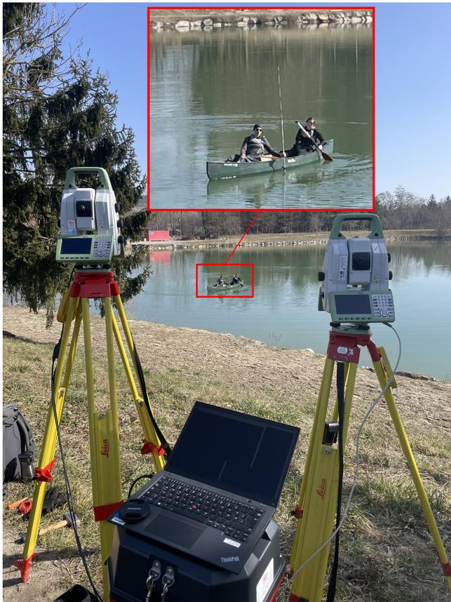
Figure 5. Photograph during data acquisition at our test site. Two Leica MS60 are controlled using a Laptop and Raspberry Pi, the bathymetric points are measured by a team of two in a canoe.
