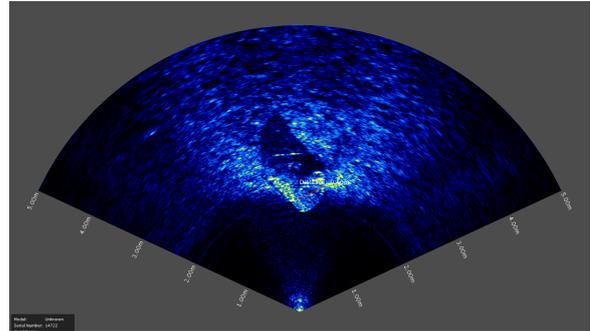
Figure 10. Barrel seen through the imaging sonar.
