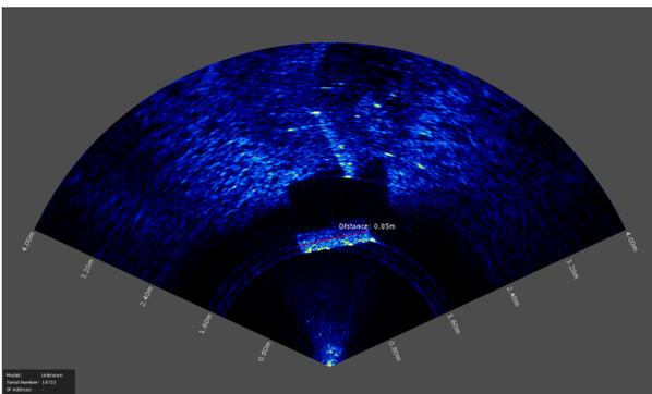
Figure 4. Barrel seen through the imaging sonar.
