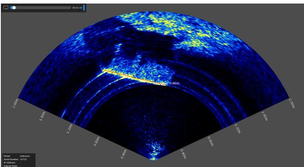
Figure 3. Barrel seen through the imaging sonar.
