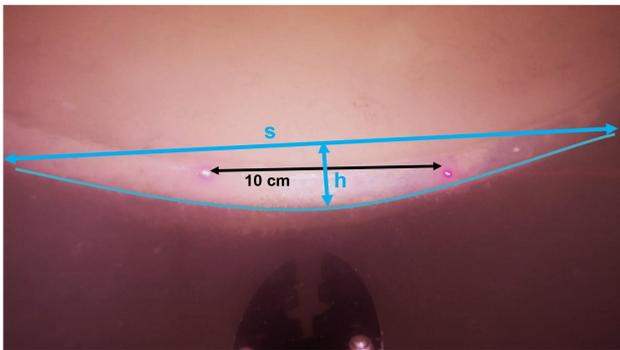
Figure 11. Part of the barrel seen in the camera. The parameters of formula (1) are highlighted in the figure.
