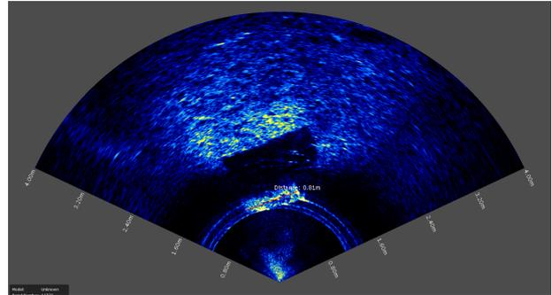
Figure 5. Barrel seen through the imaging sonar.
