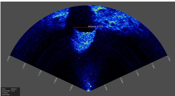
Figure 7. Barrel seen through the imaging sonar.
