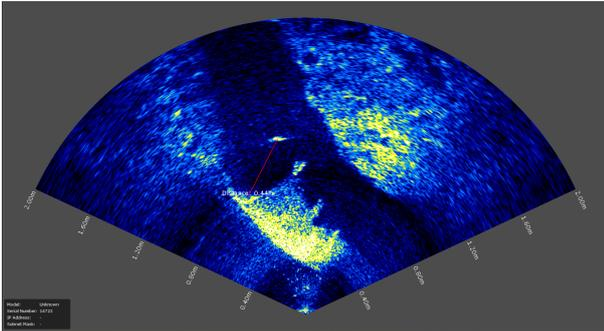
Figure 6. Barrel seen through the imaging sonar.
