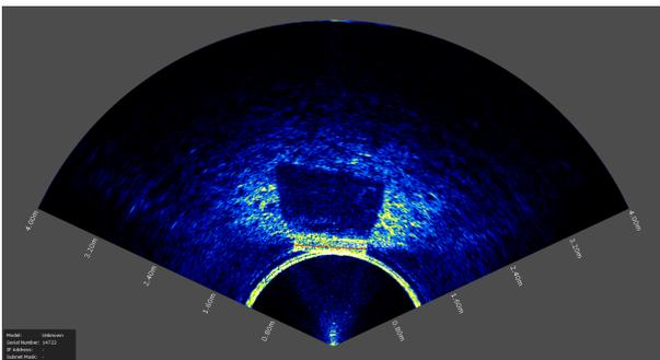
Figure 2. Barrel seen through the imaging sonar.
