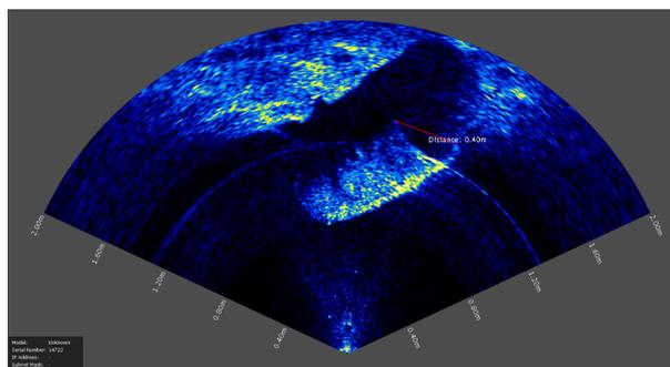
Figure 9. Barrel seen through the imaging sonar.
