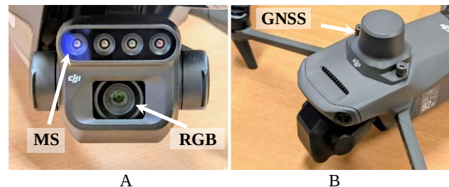
Figure 3. A: MS system, with 4 cameras, on top, and RGB camera, below. B: GNSS module on top of the drone.
