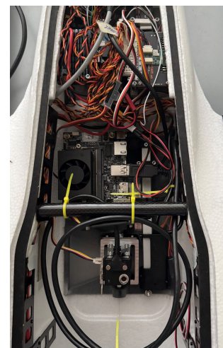
Figure 2. UAV - Internal. Bottom: Camera + IMU, Middle: Orin NX, Top: Flight Controller
