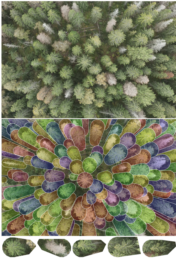
Figure 2. An example of the projection results for one image. Original image (top), segmentation based on projected cylinders (middle), and cut-out images of individual trees (bottom).
