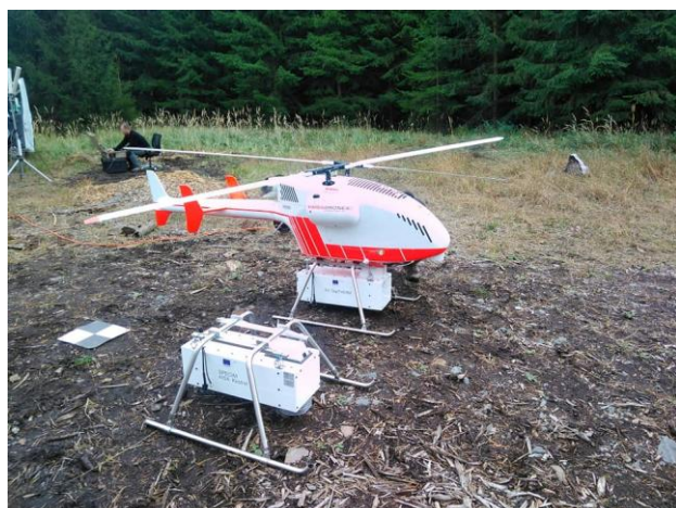
Figure 1. The SwissDrones SDO 50, a heavy-lift vertical take-off and landing unmanned helicopter used for UAV data collection in Očová and Kostelec nad Černými lesy study areas.
