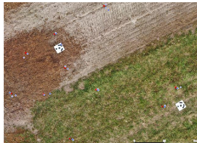
Figure 5. I-SeedChim (2X) detection locations (blue points; two repeated flights) from onboard deep-learning detection model on drone over bare soil and low vegetation coverage.
