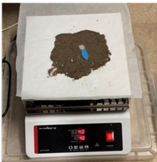
Figure 9: Use of heat plate to induce variation of temperature values for characterization of I-SeedSam Temperature sensors.
