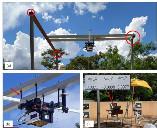
Figure 3. Laser Scanning levelling: (a) rough levelling with a bubble level, (b) refinement using the system support screws and (c) computer connected to the IMU.
