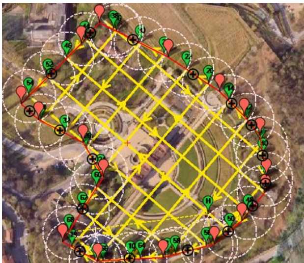
Figure 4. Flight Simulation over Villa della Regina via ArduPilot Mission Planner (2023/2024 case study)
