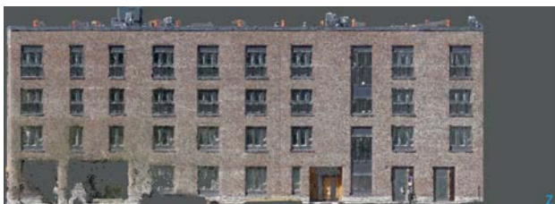
Figure 12. The photogrammetrically derived 3D point cloud of the test façade.
