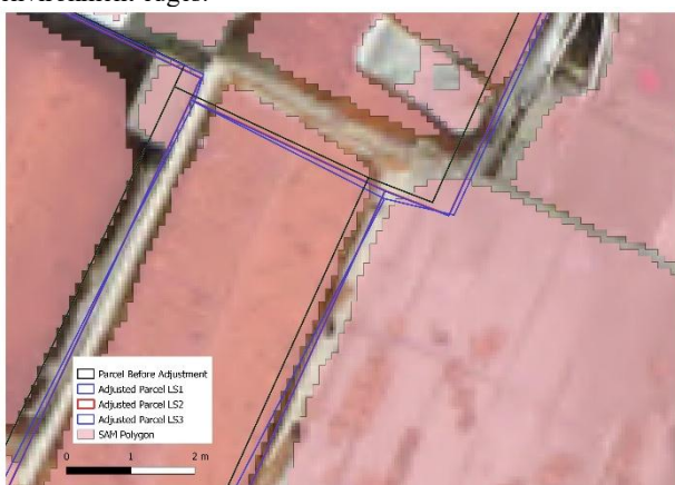
Figure 6. Overlay of original and corrected parcel boundaries (LS1–LS3) on SAM segmentation
