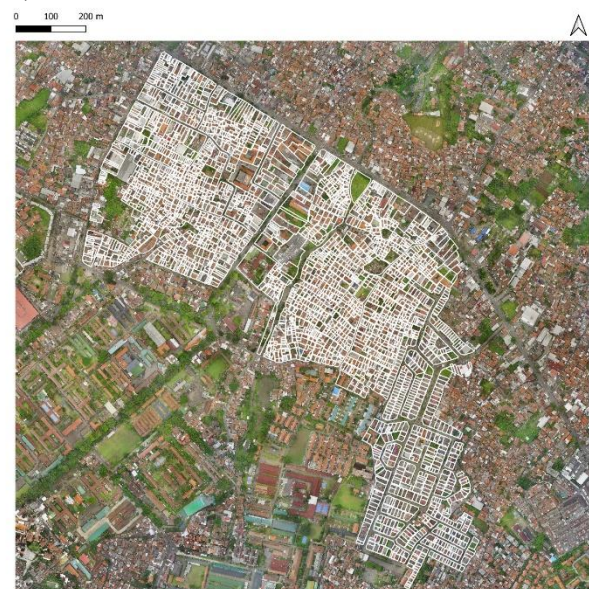
Figure 4. Overlay of cadastral parcel polygons on UAV orthophoto background in Karangmekar
