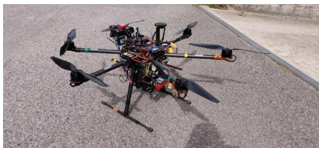
Figure 1. Custom-built UAV with a Tarot T960 frame.
