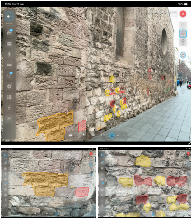
Figure 3. Real-time depth and confidence-aware reprojection of spatial annotations in the augmented reality view.
