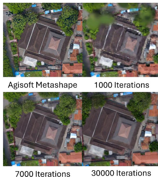
Figure 2. Visual comparison output between MVS's point clouds and 3DGS's rendered Gaussians on several iteration outputs, demonstrating progressive refinement towards photorealistic quality.
