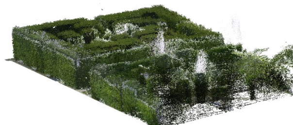
Figure 3. Point cloud acquired with the Leica RTC360 terrestrial laser scanner, showing detailed geometry of the bosquets
