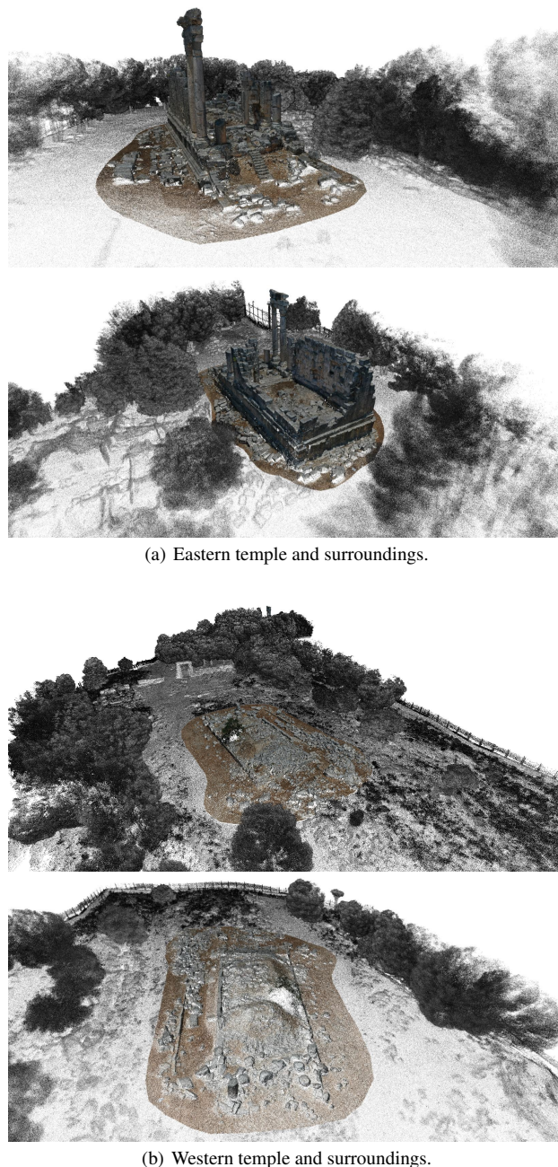
Figure 9. Integration of multi-sensor point clouds, combining close-range UAV photogrammetry for detailed temple reconstruction (shown in color) with the SLAM-based PLS dataset for full-site coverage (shown in grayscale according to intensity values).
