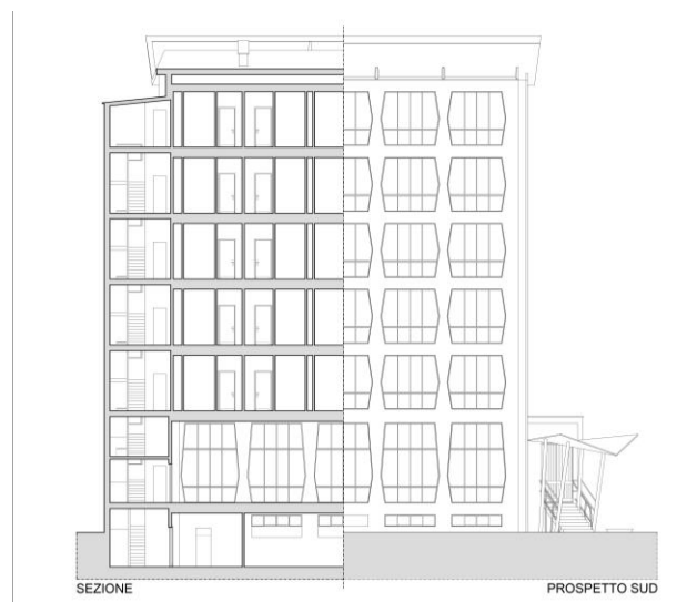
Figure 5: Section–elevation of Gio Ponti's original Institution design, reconstructed from archival documentation (original scale of the drawing 1:50).
