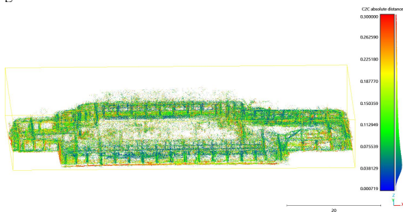
Figure 6. Cloud to Cloud Distance between TLS and 3DGS.
