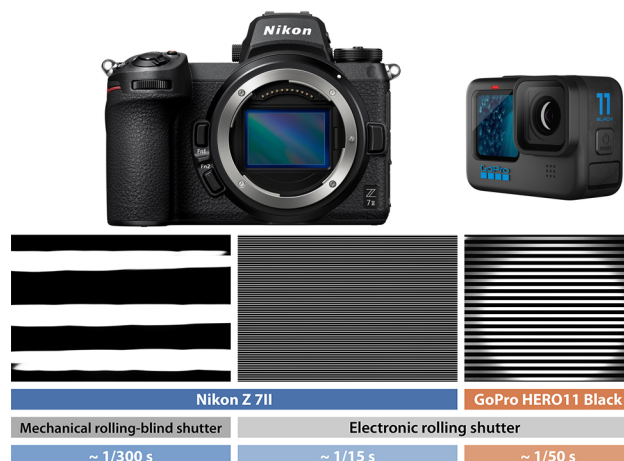
Figure 4. Estimating the transit times for the electronic focal-plane rolling shutters of the GoPro HERO11 Black and Nikon Z 7II. The latter was also tested in mechanical shutter mode.
