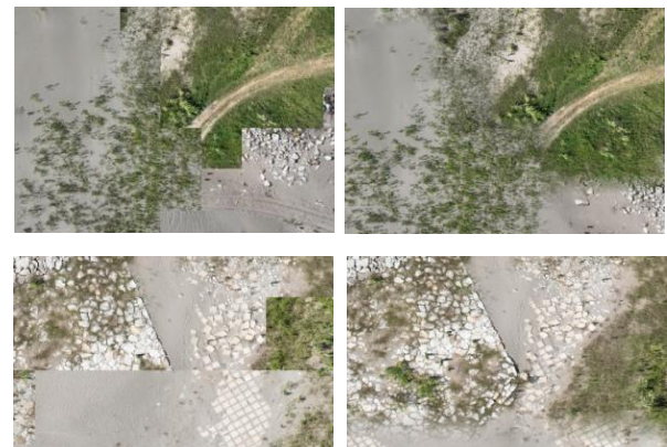
(a) Original splicing details (b) Refined splicing details Figure 5. Local DOM of 202306 data produced before and after POS refinement
