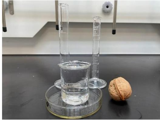
Figure 8. Set up for the nut with the WDM.
