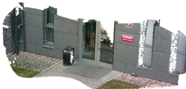
Figure 10: LiDAR point cloud coloured with the RGB camera after the estimation of the relative orientation between the sensors.
