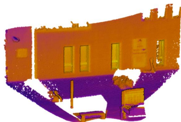
Figure 12: LiDAR point cloud coloured with the thermal camera data after the calibration process.
