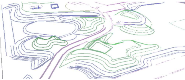
Figure 4: The 2.5D data from Gentbrugge needed for the GNSS-excavator.
