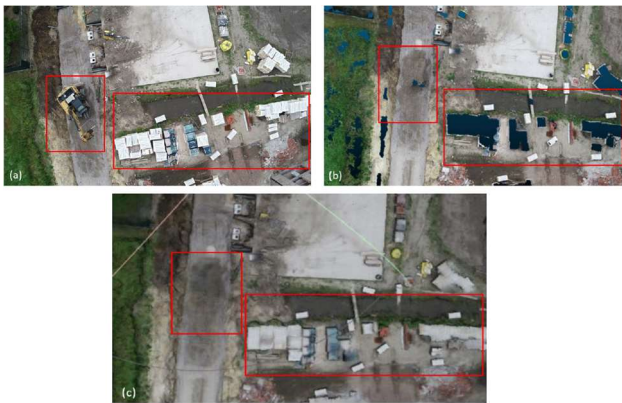
Figure 1: Problem of occlusions on construction sites. (a) Stock material and excavator seen from a georeference image. (b) The corresponding gaps in the point cloud. (c) The filled gaps in the mesh.
