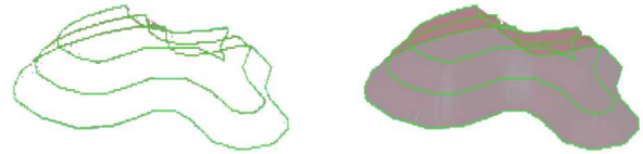
Figure 5: Converting contourlines into a 3D file for further volume calculations.
