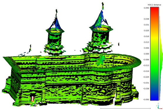
Figure 19: M3C2 distances between S2 and reference cloud.
