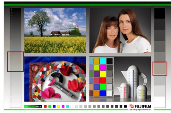
Figure 9. The result of color balance restoration based on averaged correction values at 32 pixel bit intervals.
