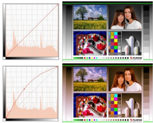
Figure 5. Artificial color balance disturbance in red color component using a Fujifilm Test Image.
