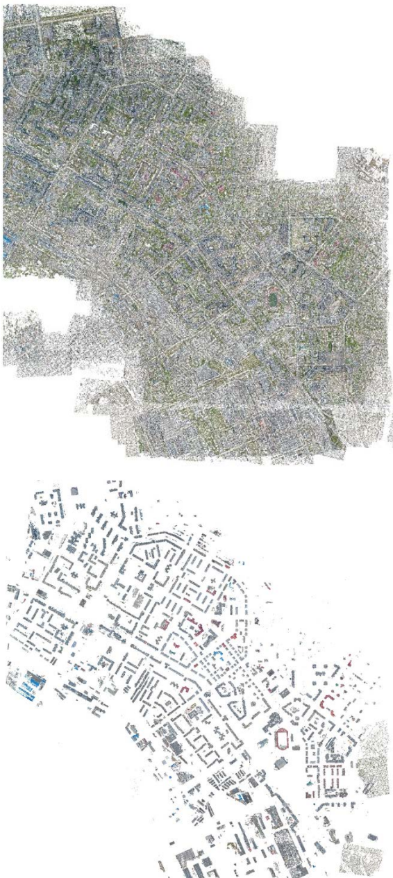
Figure 9. Sample of tie points clouds without (up) and with (down) masking.
