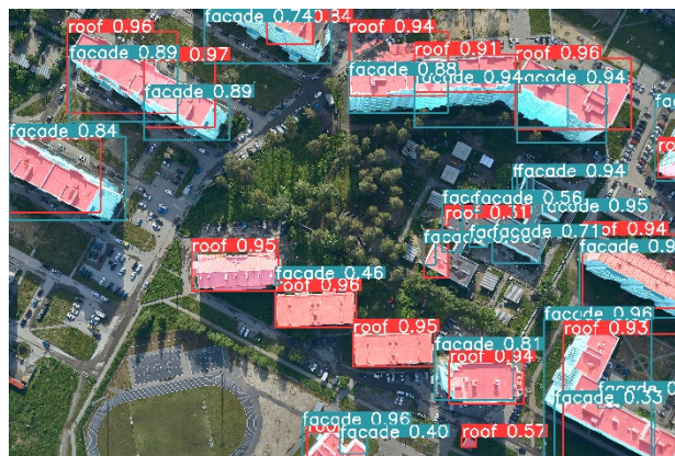
Figure 5. Sample of a mask for roofs and facades with classes
