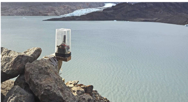
Figure 8. SAGAZ monitoring station in the Laguna Frías superior with a prototype lake level sensor with GNSS-IR technology (Photo by Camilo Rada).
