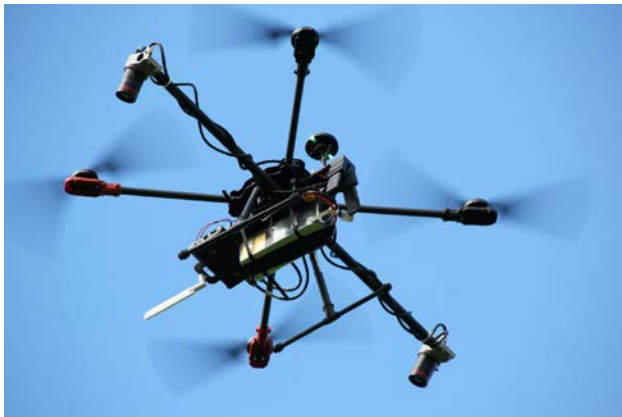
Figure 1: UAV used in the REALTIME3D system, equipped with stereo cameras.
