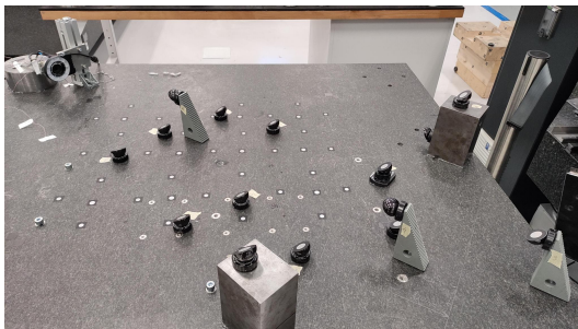
Figure 1. Experimental set-up: granite table, camera-lens system, light source, optical circular retroreflective markers (hemispheres) and support structures.
