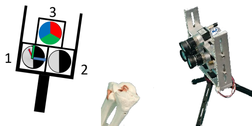
Figure 3. Setup of the trinocular camera (left, (Kahmen et al. 2020)) and when aligned with an anatomical knee model (right, (Schierbaum et al. 2024))
