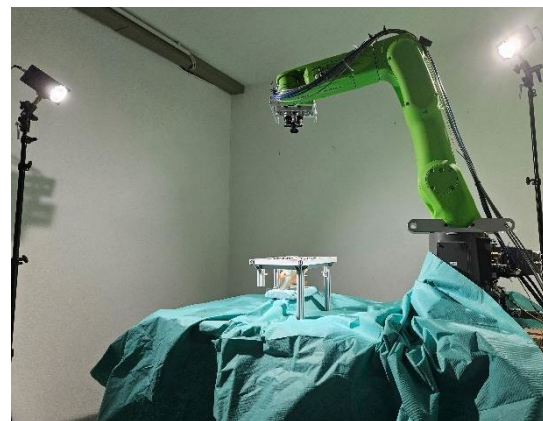
Figure 6. Experimental setup with the robot and the artificial knee joint surrounded by the reference frame with two spotlights from opposite sides
