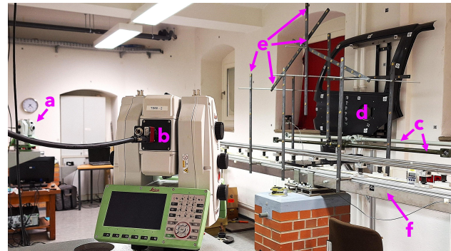
Figure 8. Experimental setup with TS60-1 (a) and TS60-2 (b) (each equipped with a Guppy camera), subtense bars (c) for the base line determination, car door for experiment 2 (d), additional structure for experiment 3 (e) and the mounting rail (f).
