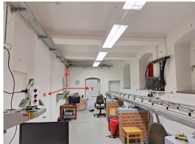
Figure 1. Setup of the two total stations TS60-1 (A), TS60-2 (B) and the observed objects in the geodetic measurement lab at TU Dresden. The origin of the right-handed coordinate system lies in TS60-1 and the x-axis points towards TS60-2 after the baseline determination using exact collimation.
