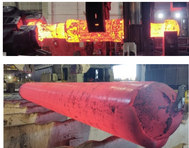
Figure 6. Early stage of shaping (upper part) and final stage of forging (lower part).
