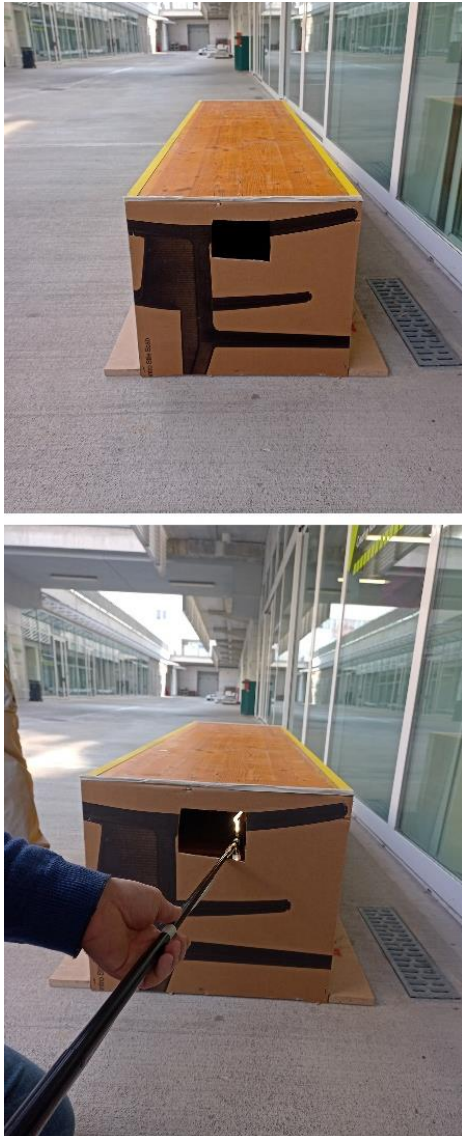
Figure 7. The wooden box used for the experiments (top) and the insertion of the boroscope (bottom).
