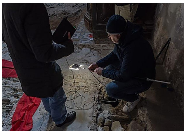
Figure 2. The remote connection allows 360° inspection and data acquisition with real-time visualization.
