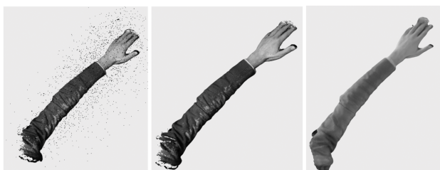
Figure 4. Example of result cloud (left) post-processing (center) and meshing (right).
