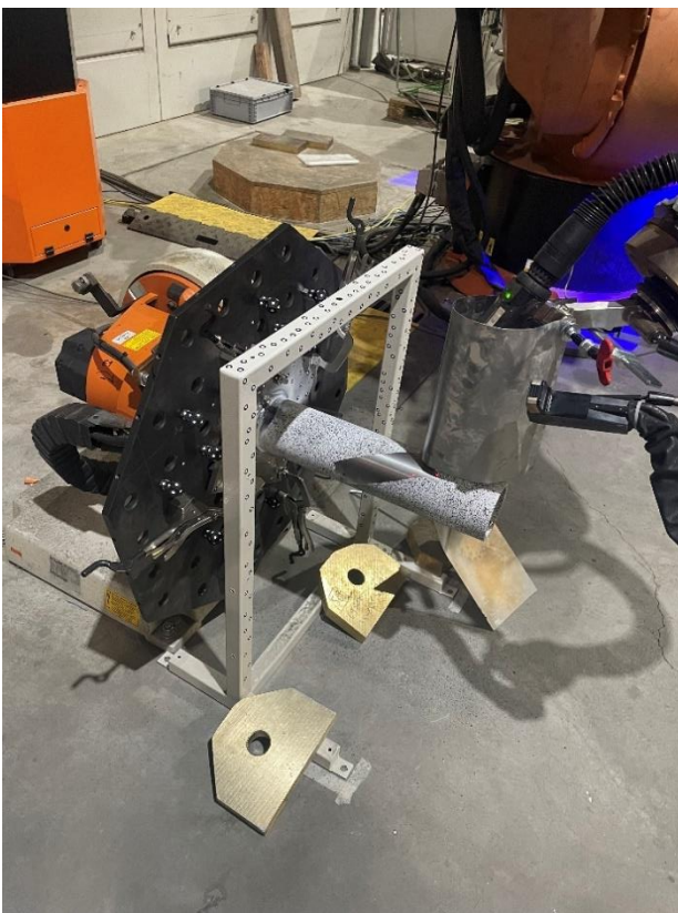
Figure 3: Welding rig prepared for the monitoring (Hack, D.)
