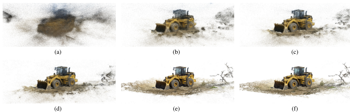
Figure 6. Extracted point clouds for the Caterpillar scene at steps s : (a) 78, (b) 240, (c) 499, (d) 1073, (e) 10123, (f) 29999. Subfigure (f) shows the point cloud after the last training step.
