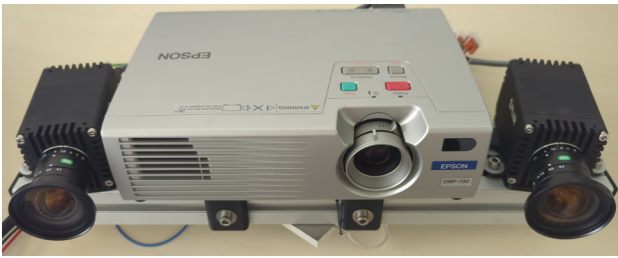
Figure 4. Experimental stereo camera system with mounted projector.
