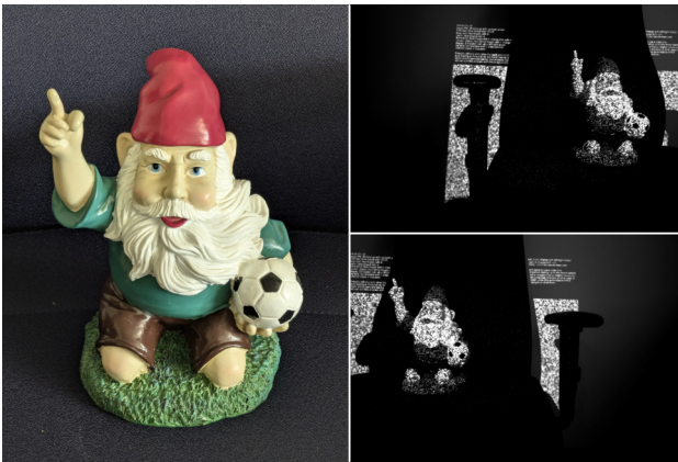
Figure 12. The garden gnome reference object. Left: overview of the gnome placed on a chair. Right: input stereo image pair (enhanced contrast for display).
