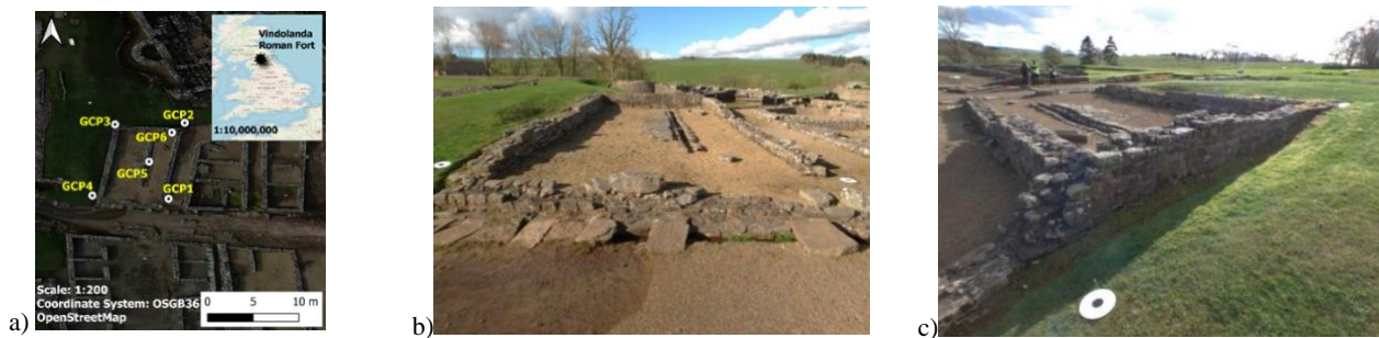
Figure 1. (a) Test field target distribution around Vindolanda Roman Fort study area visualized on an orthoimage generated with a DJI Phantom 4 RTK. (b, c) Example imagery captured using the GS18i of the study area, including GCP/ICP targets.
