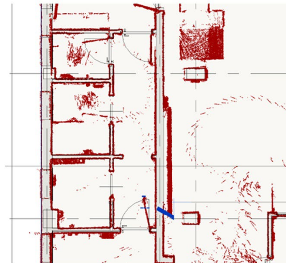
Figure 2. Model in BIM environment from a point cloud made with Leica BLK2GO mobile laser scanning station
