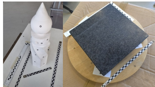
Figure 2. Structure of the recording object with calibrated scale bars around it for scaling the image data and the 3D model to be created.
