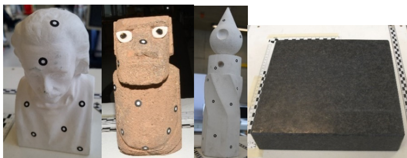
Figure 1. Reference bodies for the benchmarking test (f.l.t.r.) – Einstein bust, Moai figure, Testy, and planar granite slab.
