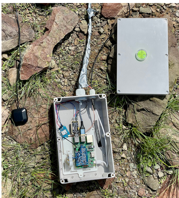
Figure 7. Raspberry Shake system mounted in waterproof enclosure, with GNSS antenna connected (left) and bubble level mounted to the lid (right).
