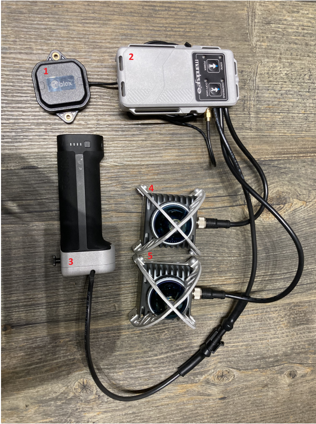
Figure 1. Re-configurable mobile mapping system - all main components. 1: GNSS antenna, 2: data collection unit, 3: battery, 4 and 5: LiDAR LIVOX MID 360.
