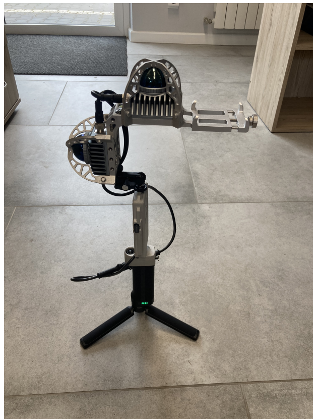
Figure 4. Configuration 4: Hand held mobile mapping system.
