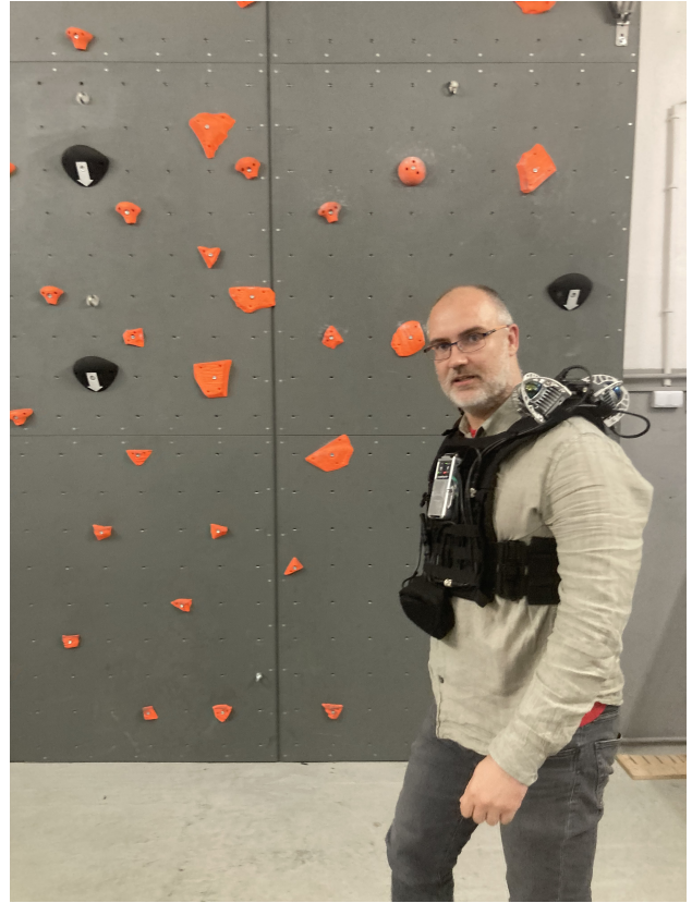
Figure 2. Configuration 1: Mobile mapping system mounted on the shoulder.
