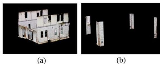
Figure 15. Point cloud data of corner sections.
