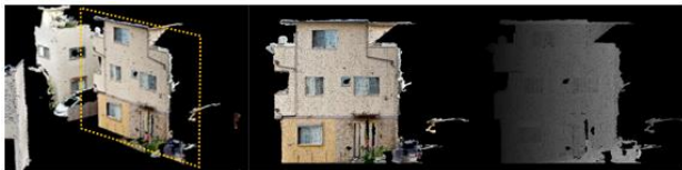
Figure 6. Projected 2D point cloud image
