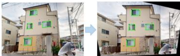
Figure 7. Wall frontalization via homography
