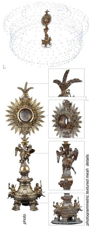
Figure 3. Comparison between photo and 3D photogrammetric model: despite the high level of detail, there are gaps on smooth surface of the golden globe.
