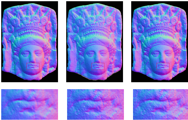
Figure 10. Three normal fields of the Cypriot head represented in false colors. Left column: photogrammetry result obtained with the Metashape software. Center column: calibrated PS result obtained with an RTI dome. Right column: result obtained with the new PS method we propose. The bottom line shows enlargements of an area located at the mouth.
