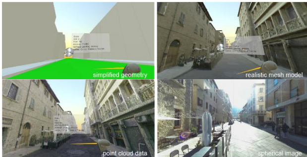
Figure 4. Four different representation methods in the VR view.
