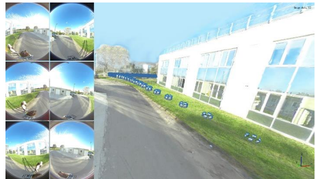
Figure 8. A 3D view of the photogrammetric survey in a portion of the campus.
