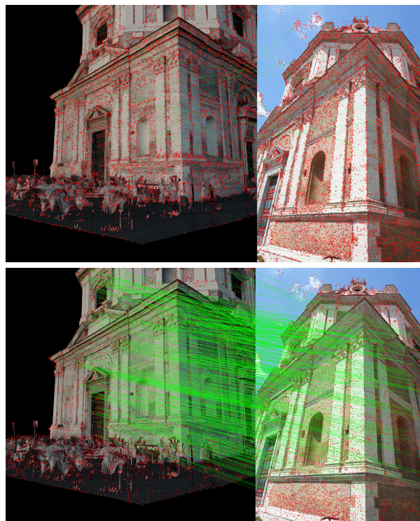
Figure 6: Matches (green lines) between TLS renders and RGB images with RootSIFT (top) & SuperPoint+LightGlue (bottom).
