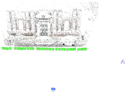
Figure 4: Camera network for the Santa Maria di Loreto dataset. RGB camera poses in green, positions of TLS renders in blue.
