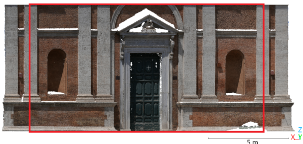
Figure 7: The area of the façade used for the accuracy evaluation. Results are reported for the entire areas shown in the figure and for just the area inside the red rectangle.
