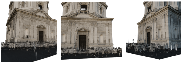
Figure 3: Rendered images from the TLS point clouds using only the intensity values from the TLS data.
