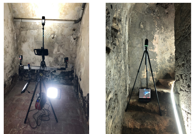
Figure 6. Photogrammetric acquisition in the cell (left) and lasergrammetric station in the tunnel (right).
