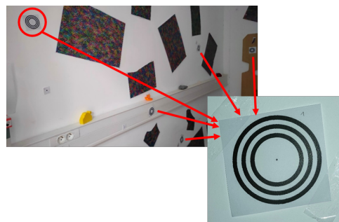
Figure 2. Test subject's wall with random patterns and CCTAG3s network.
