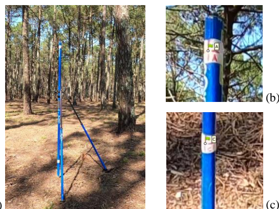
Figure 4. Surveying pole, supported by a bipod (a), and marks in the top (b) and bottom (c) of the pole.
