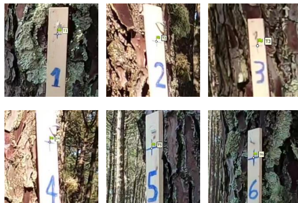
Figure 6. Check points surveyed with a total station to assess the positional accuracy of data extracted.
