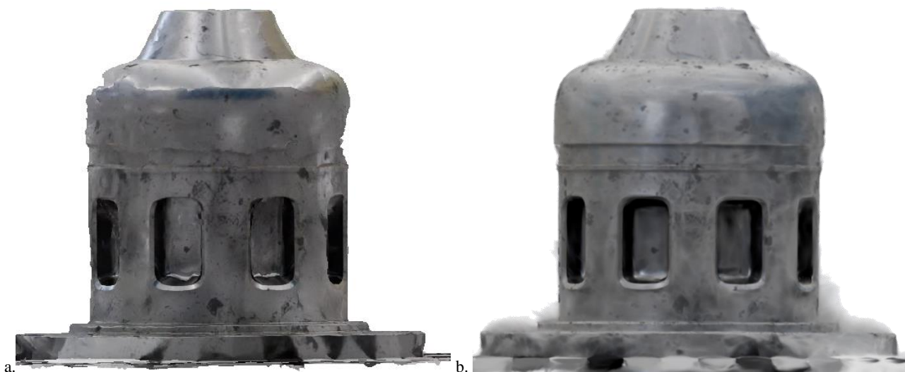
Figure 4. Comparison of orthophotos for the "mechanical" datasets: a) "standard" approach results (see artefact in the top part of the element) and "gaussian splatting result".
