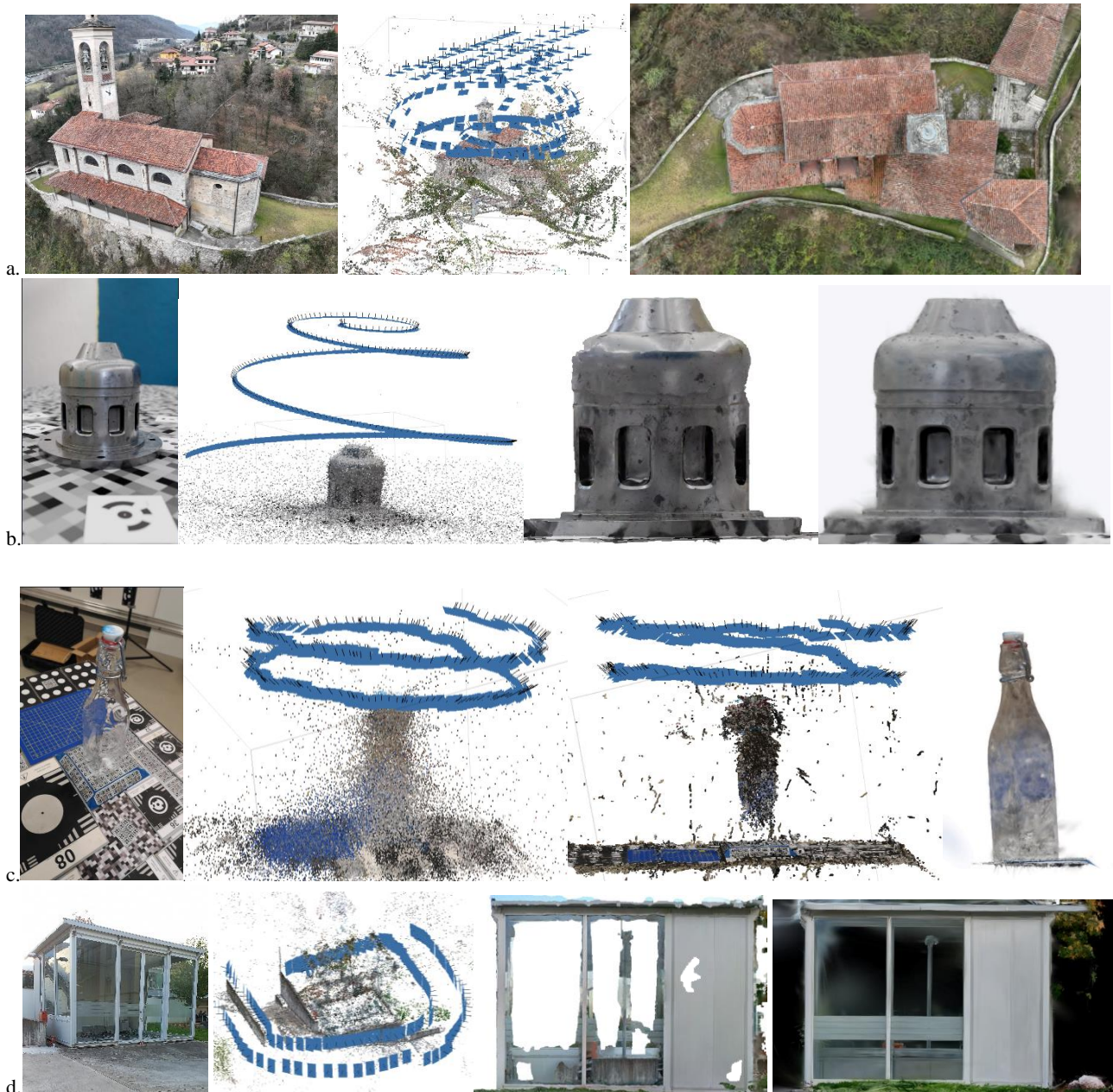
Figure 3. Results of orthophoto derived from gaussian splatting models: a) “San Michele” dataset (from left to right: image of the dataset, orientation results, gaussian splatting orthophoto results); b) “Synthetic Metallic” dataset (from left to right: image of the dataset, orientation results, orthophoto from standard approach, and orthophoto from gaussian splatting approach); c) “Bottle” dataset (from left to right: image of the dataset, orientation results, dense clods reconstruction results, gaussian splatting orthophoto results); and d). “Architectural Glass Case” dataset (from left to right: image of the dataset, orientation results, orthophoto from standard approach, and orthophoto from gaussian splatting approach)
